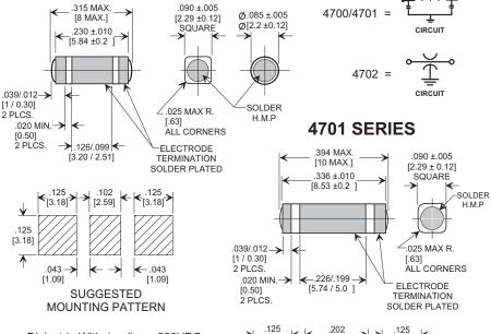
Dielectric Withstanding - 300VDC Direct Current Rating - 10 ADC Inductance Value - 100nH Minimum
